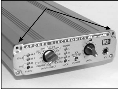
1. Remove the two TOP screws from the Mini-DAC front panel, using a 1/16" hex wrench.
