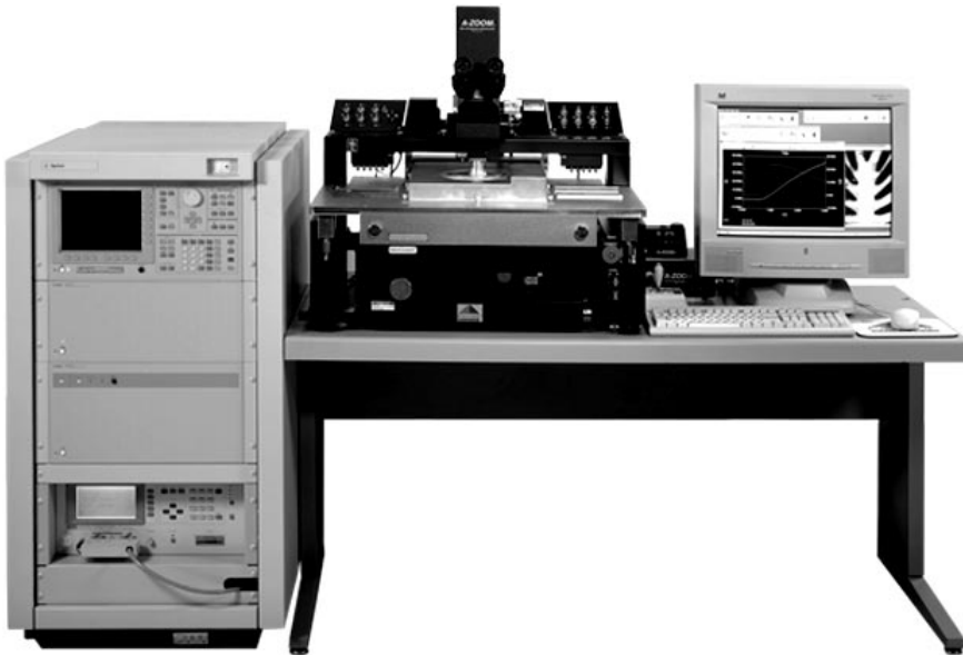
Figure 1. Agilent 4156C, 4284A, and E5250A with wafer prober
