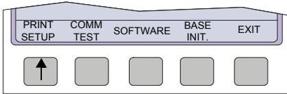
→ To obtain a printout press the PRINT SETUP softkey.
