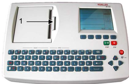
1. Press the locking catch (1) to the right. Open the printer door opens upward.
