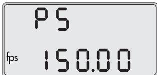
Note: The frame rate can be set between 0.1 and 150 fps. For frame rates over 130 fps and a ramping speed set to LO or St, the power supply voltage has to be at least 24 V. for rampspeed Hi at least 26.5 V.
