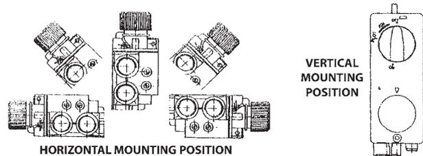
Main gas NPT connections (inlet or outlet)
