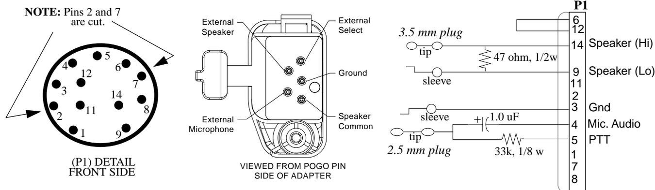
**NOTE:** For proper speaker impedance, the RTX4005B test set *Audio out* switch must be set to the “MX” position
