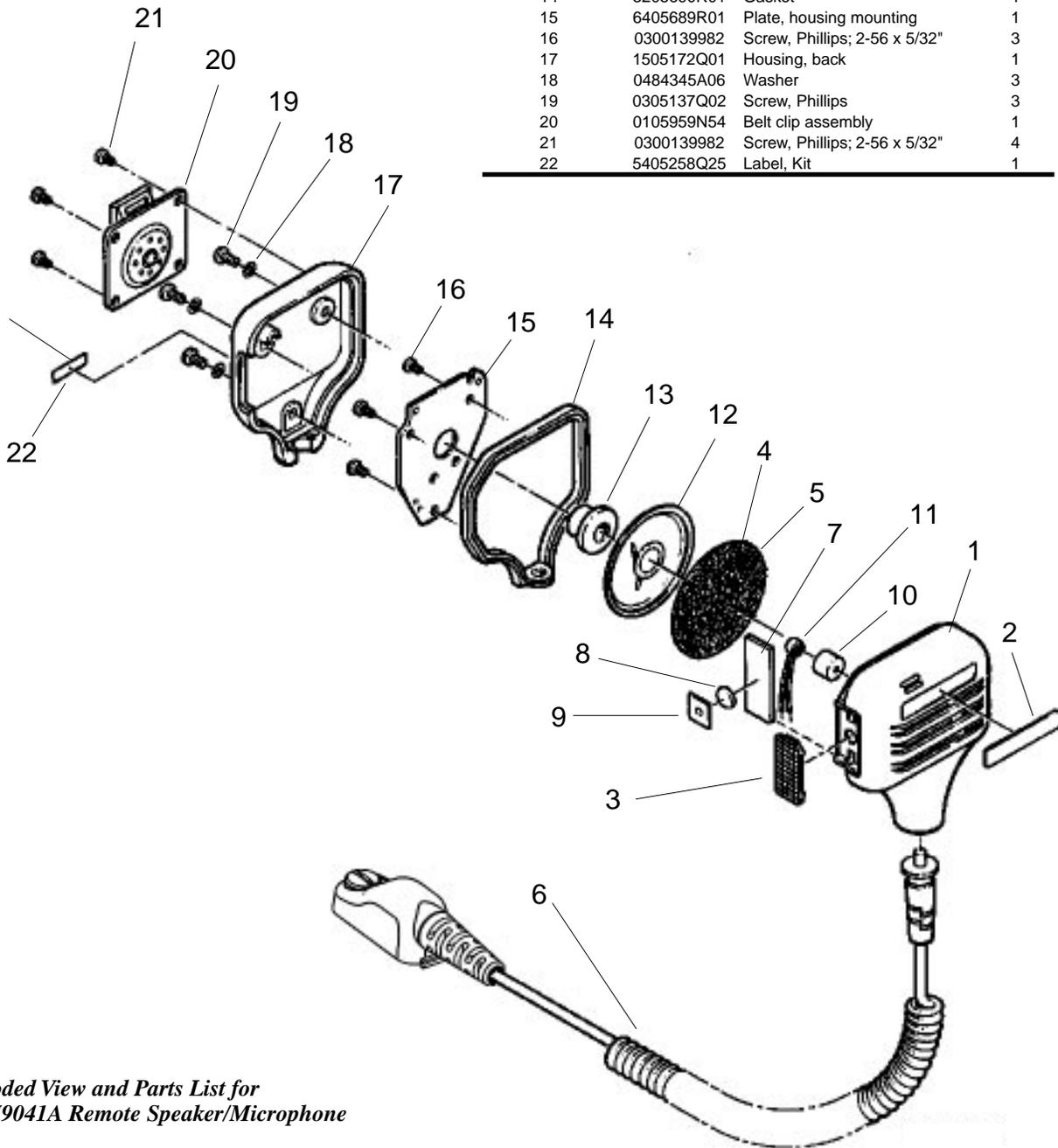
*Exploded View and Parts List for HMN9041A Remote Speaker/Microphone*
