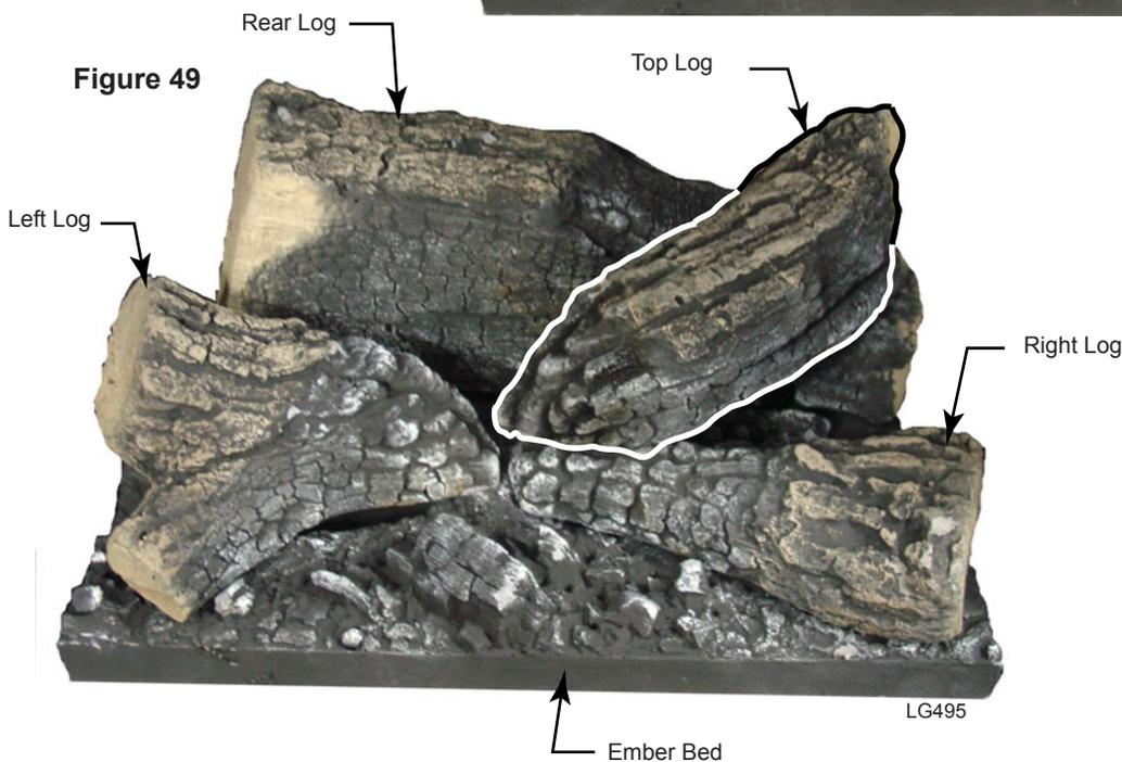
5. Install top log by mating hole on bottom of log with locating pin on top right side of rear log. (Fig. 49) Position log so it is angled down toward the area where the front two logs meet.
