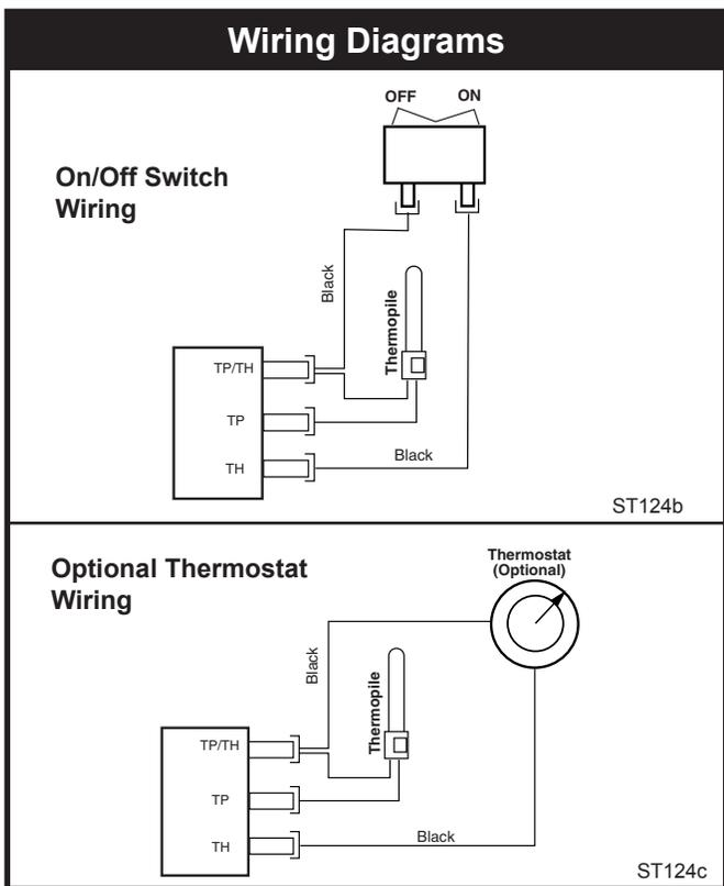
Fig. 79 On/Off switch and optional thermostat circuit.
