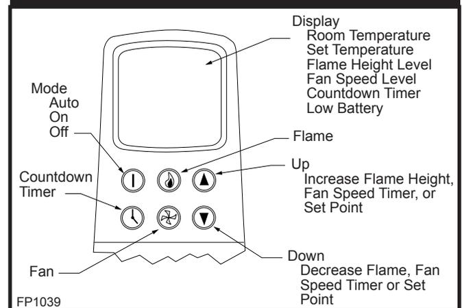
Fig. 57 Transmitter diagram.
