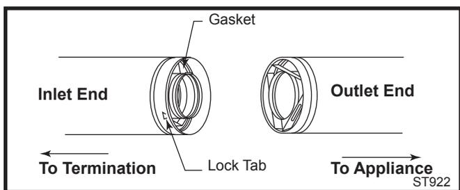
Fig. 33 Joint connection.
