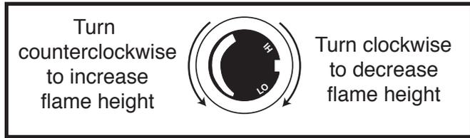
Fig. 54 Flame adjustment knob for SIT valve.
