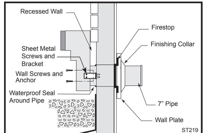
Fig. 30 Use extension brackets to mount snorkel against recessed wall.
