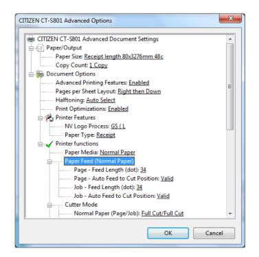
\*If Auto Feed to Cut Position is set for valid and Feed Length is specified, paper feed to cut position is done first then specified paper feed is performed.
