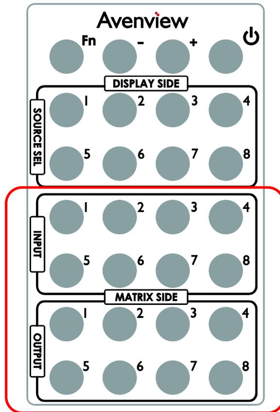
Choose the output port you want to make channel switch from OUT1 to OUT4 then press 1-4 channel button to choose the HDMI input source shown on the chosen output display.
