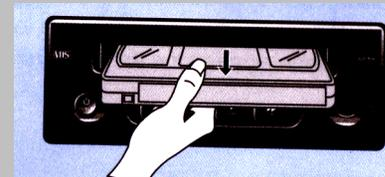
When you press the STOP/EJECT key even if the power is off, the cassette will be ejected.
