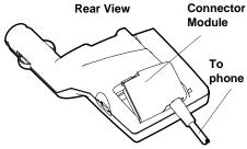
2. Tilt the connector module upright, insert the hook into the mating slot, then press down to secure it in place.
