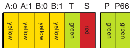
Figure 2-5. LED Labels and Colors GDT8546RZ
