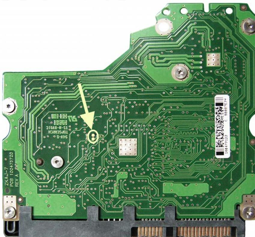
Fig. 38. Board view from the external side. Connection points are marked in yellow.
