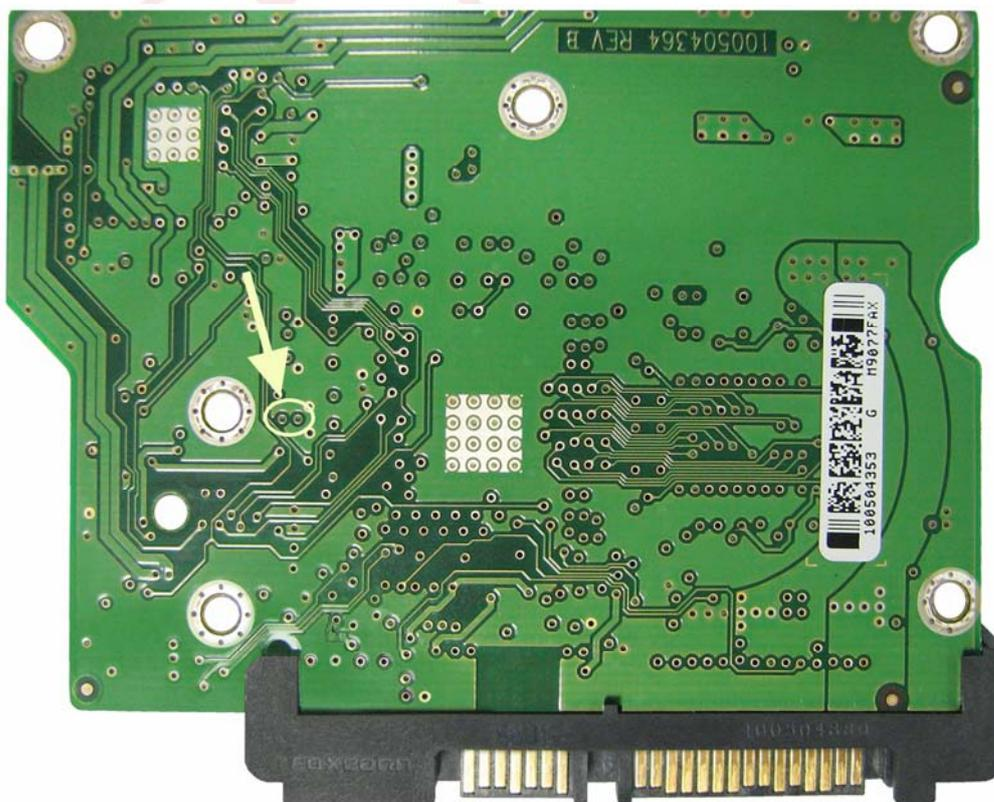
Fig. 34. Board view from the external side. Connection points are marked in yellow.
