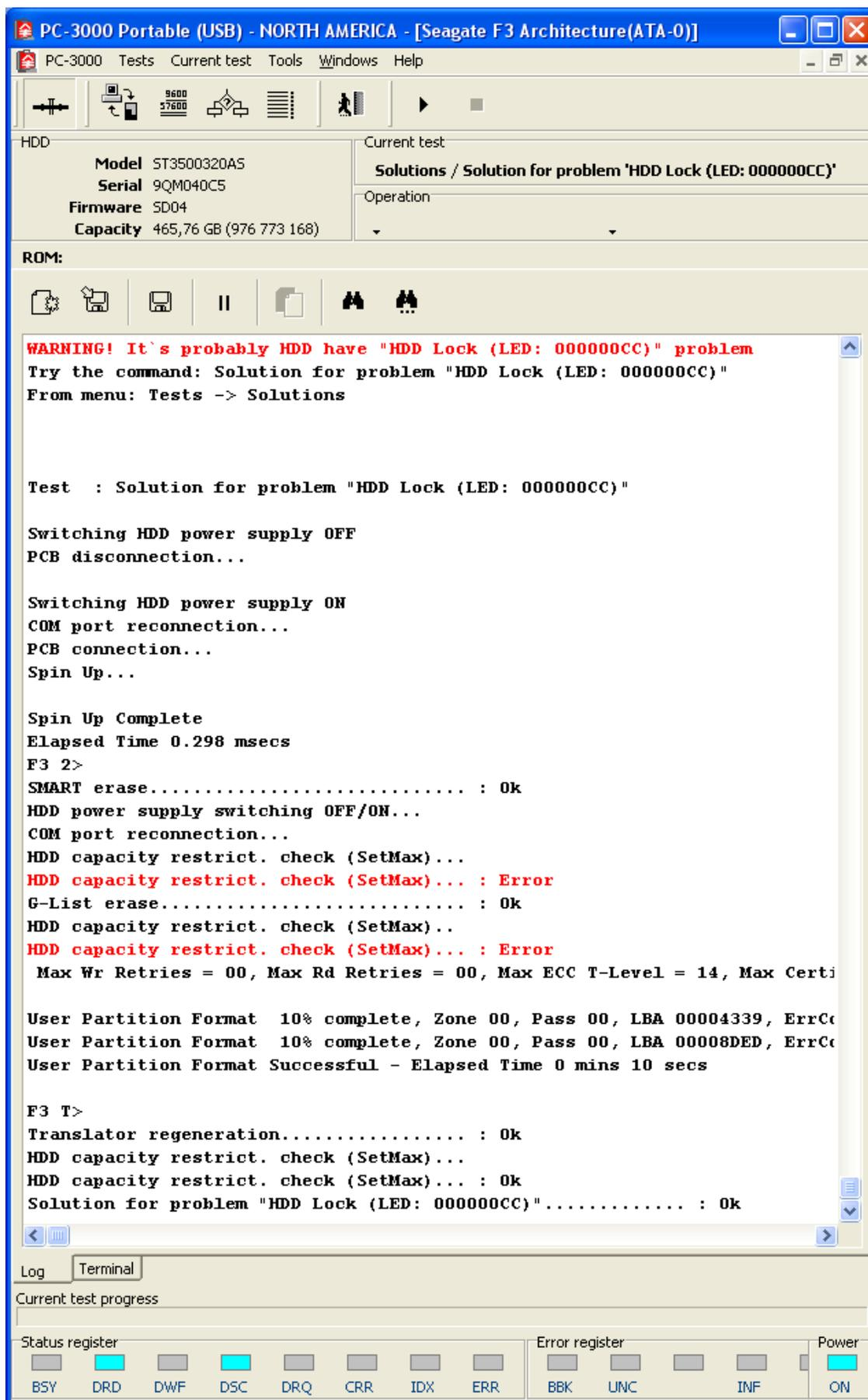
Fig. 17. Log of the unlocking procedure.
