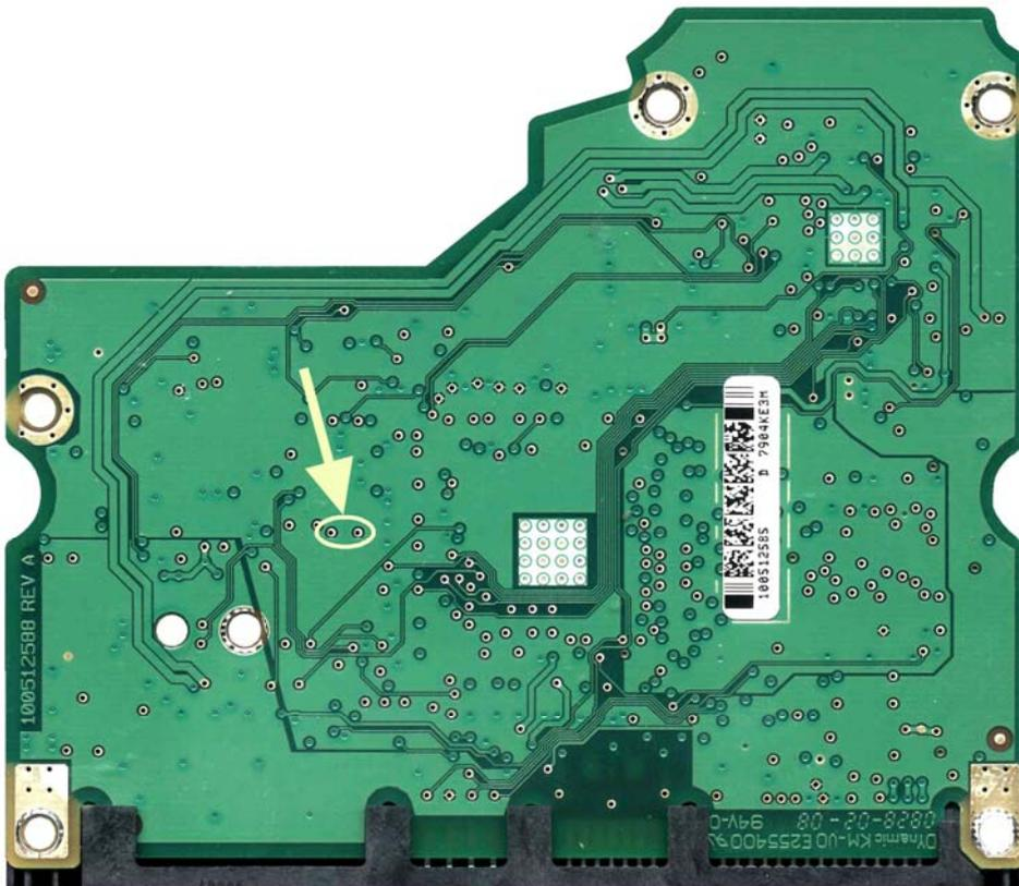
Fig. 36. Board view from the external side. Connection points are marked in yellow.
