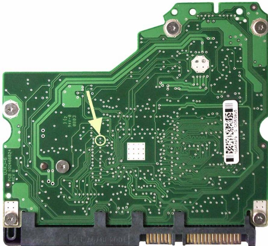
Fig. 28. Board view from the external side. Connection points are marked in yellow.
