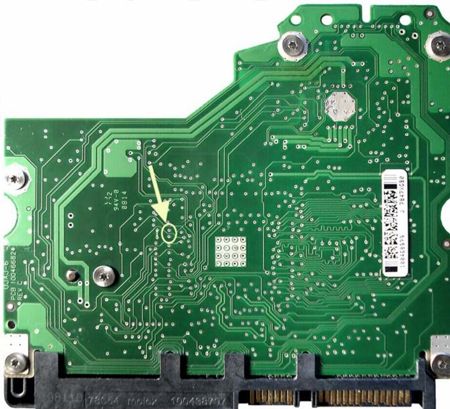
Fig. 30. Board view from the external side. Connection points are marked in yellow.
