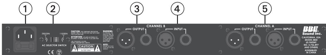
1. AC POWER CORD INLET: Plugs into AC power receptacle. U.S., Canada and Japan Models, 100-120Vac, 50/60Hz. All other models, 220~240Vac, 50/60Hz.
