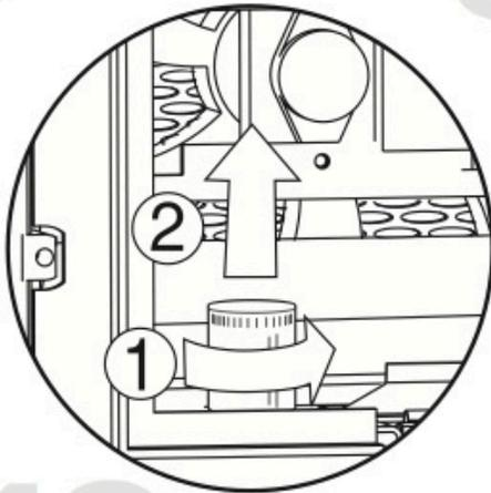
10. Rotate starter and lift to remove.
