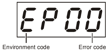
Figure 3-2 Example GENERAL STATUS LED (no error)
