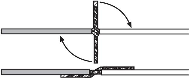
4. Use electrical tape to wrap, be sure to cover about 2 inches on either side of connection. Secure with wire ties as shown.
