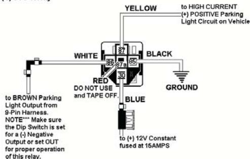
(-) Negative HIGH-CURRENT Parking Light Output using (1) 775 Relay
