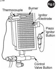
2A. Alternatively, hold a lit taper to the **burner face** while pressing and holding the control valve button. After the burner ignites, keep button pressed for one (1) minute or until the burner stays lit after releasing button.
