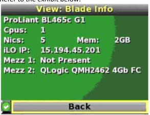
A customer reports that Insight Display shows five NICs installed in a half-height server blade, but a connection to only two of them can be established. What could cause this to happen?
