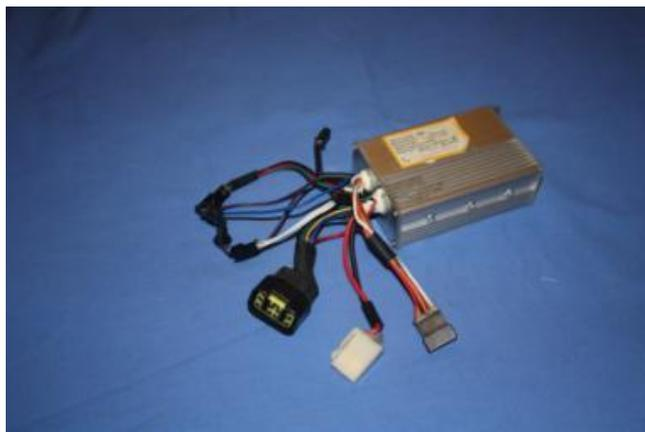
2008-2009 type controller with multi-pin motor connector
