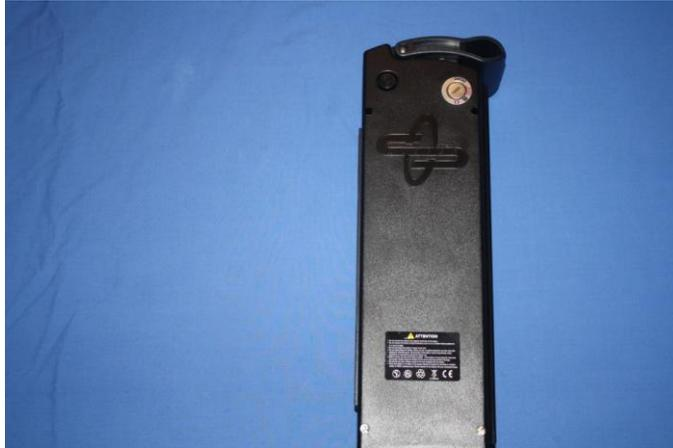
2. The fuse fitted at the top of the battery next to the key switch is the charging fuse and is rated at 5 amps.
