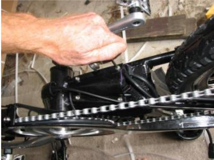
4. Unplug the eight-pin motor cable plug or the 3 separate motor connectors and one 5-pin connector.
