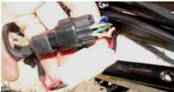
5. Note: depress the end of the release lever to unlock the plug so you can disconnect it.
