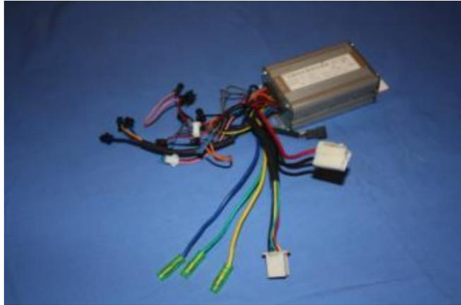
Early 2008 model controller with separate motor connectors
