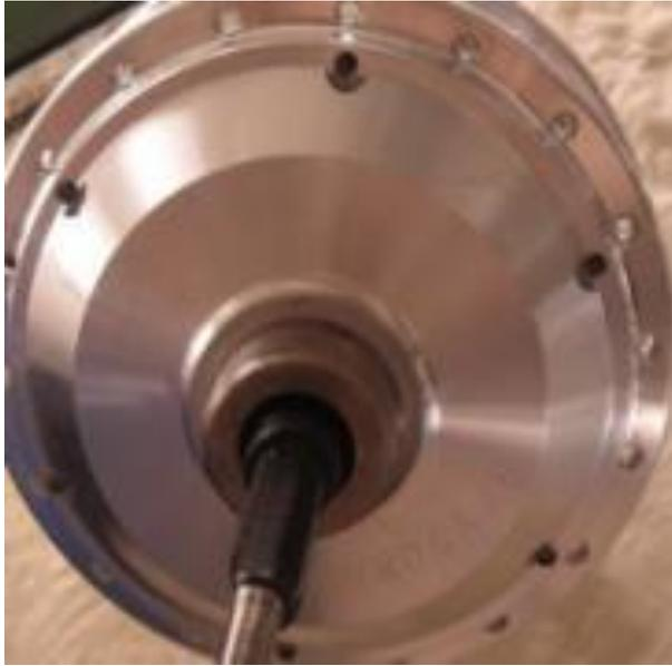
8. Take off the left hand nut that keeps the entire inner assembly in the hub.
