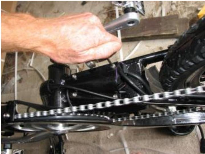
4. Unplug both the eight pin motor cable plug and the two pin battery input plug.
