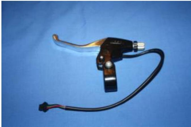
2008 onwards using a 3-wire type switch
