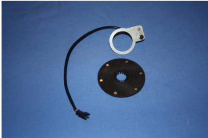
2. The assembly comprises a disc containing 5 or 6 magnets that is fitted to the bottom bracket axle and rotates with the pedal cranks, and a fixed sensor fitted to the frame.
