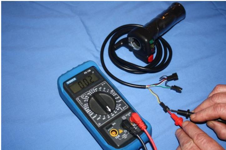
10. No other testing of throttles apart from checking connections is practical without more specialised equipment and they should be replaced with genuine Wisper parts if found faulty following correct diagnosis procedures in the fault finding sections 7 and 8.
