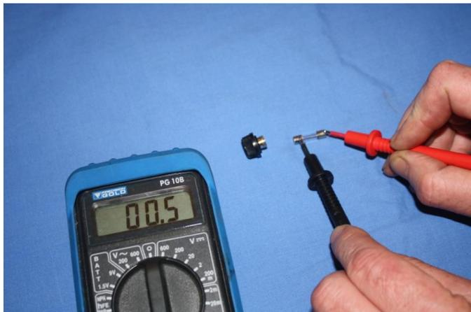
10. A reading of close to 0 Ohms should be obtained on the meter. If higher this indicates a poor contact or blown fuse which should be replaced using a genuine Wisper replacement fuse only of the correct capacity. Check the end caps are secure on the fuse before refitting and if in doubt replace the fuse.
