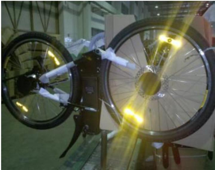
2. From the underside remove the tunnel shaped cover by unscrewing the 4 Allen screws holding the bottom cover in place (it is the tunnel shaped plate, just behind the pedal crank axle – on the bottom of the bike, directly under the battery/controller housing).
