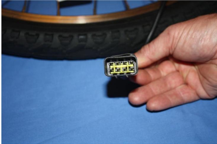
16. Always ensure the colour codes on the 8 motor cables match the corresponding colours on the controller connector and that the power connectors are not swapped with the Hall effect connectors. Regular maintenance for bikes fitted with an eight way multi-pin connector is recommended. Further details are included in section 11.
