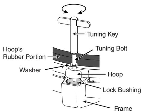
\* The lock bushings prevent rotation and loosening of the tuning bolts caused by vibrations that are transmitted from the hoop as you play.
