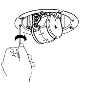
Power the dome (heater fans turn on). The camera lens then follows a pattern until it reaches its home position. The controller can then be used to call up and control the dome.
