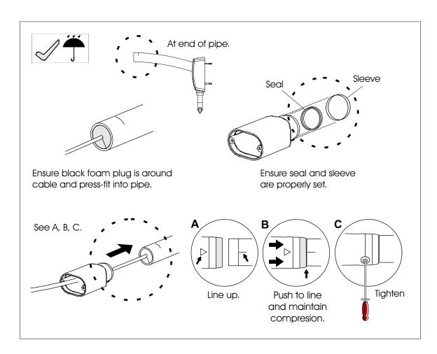
Thread cables through end cap assembly and attach housing to mounting structure.
