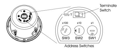
The camera/motor assembly is shipped "terminated" (switch to left) for when it is installed at the end of a data cable. Should the cable continue to another dome, move the slide switch to the right to "unterminate".
