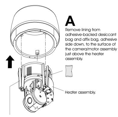
Align the three arms of the chassis over the tabs inside the sunshield of the housing.
