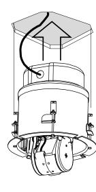
Turn each of the four locking screws clockwise to seat the "swing out" mounting clips tightly against the ceiling.
