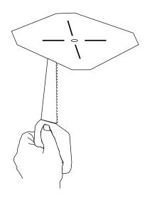
Adjust all four "swing out" mounting clips for the ceiling thickness.
