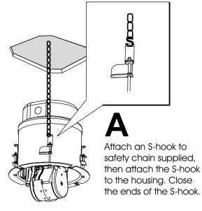
Secure the housing to the ceiling.
