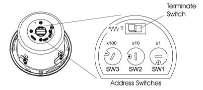
The camera/motor assembly is shipped "terminated" (switch to left) for when it is installed at the end of a data cable. Should the cable continue to another dome, move the slide switch to the right to "unterminate".
