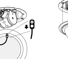
Turn the bubble clockwise until it catches the tabs and
