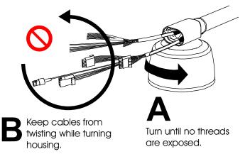
Attach cable connectors (in kit 0351-1686-01).
