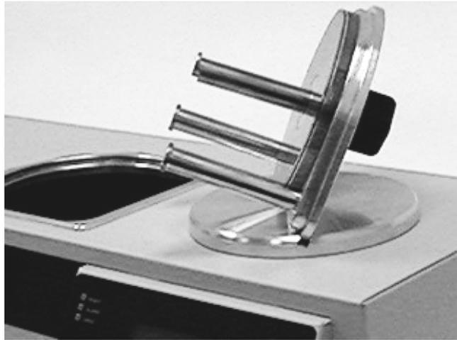
2. Unscrew the handle from the back of the holder and remove the **Center Spindle**.
