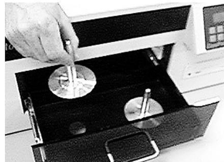
**Output Spindle**      **Reject Spindle**
