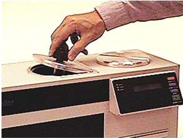
Note: With the **Input Spindle** in place, the label sides of the discs face up
