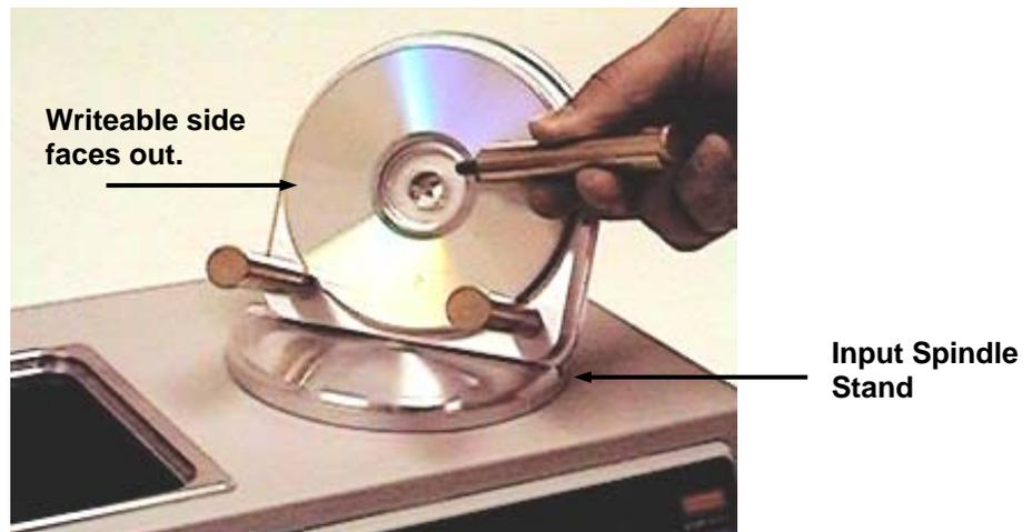
3. Place blank CD-R discs on to the **Input Spindle** writeable side out (away from the back plate) as shown.
