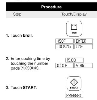
When the oven reaches the programmed temperature, a signal will sound 1 time.
