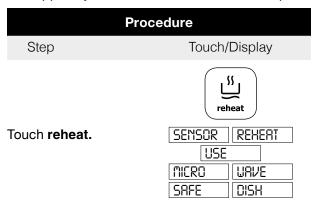
Microwave starts automatically. When the sensor detects the vapor emitted from the food, remainder of cooking time will appear.
