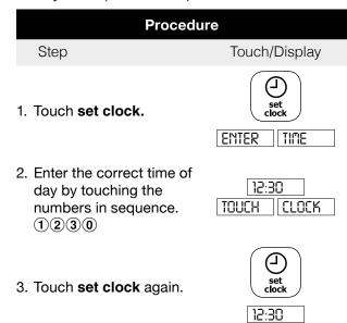
This is a 12 hour clock. If you attempt to enter an incorrect clock time, *ERROR* will appear in the display. Touch the **STOP/CLEAR** pad and re-enter the time.
