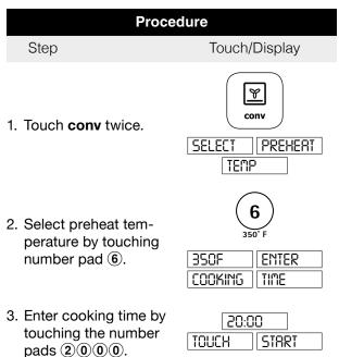
When the oven reaches the programmed temperature, a signal will sound 1 time. The oven will stop, and directions will be displayed. Follow the indicated message.
