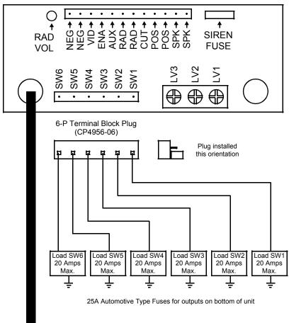
Supplied with #10 AWG RED Internal screw pressure terminal will accept up to #6 AWG for input current higher than 40 Amps
