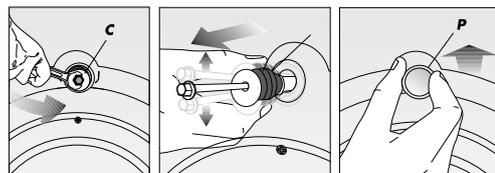
1. Loosen "C" bolts by rotating them counter clockwise with a suitable spanner
