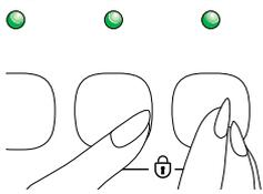
**Function Selection:** Depending on the selected program, the selectable auxiliary functions are selected by pressing the each function’s button. The light of the selected function comes on. Since it is not possible to select some of the auxiliary functions together, one of them becomes off when the other one is selected.
