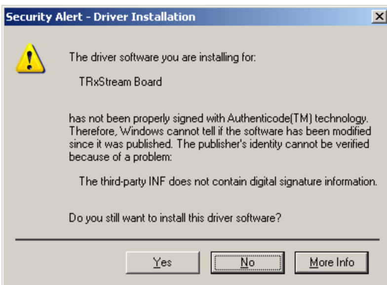
Screenshot 4: Confirm installation of unsigned drivers
