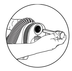
(2) Pull the crevice tool out of the base of the cleaner.
