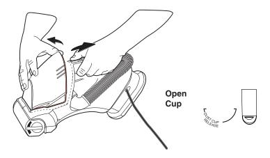
Pull back on the power switch to the "open cup" position and lift dust cup away from cleaner.
