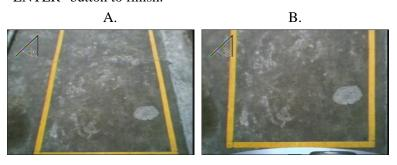
9) After you finish the Angle Setting there should be an "ON/OFF" icon in the top corner of your screen. Take the vehicle out of reverse gear so the camera shuts down. Wait 2 seconds and then put the vehicle back into reverse gear. You should see an hour glass as all the changes are loaded.
