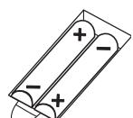
2. Place the batteries in the compartment as indicated by the polarity symbols (+ and -) marked inside.
