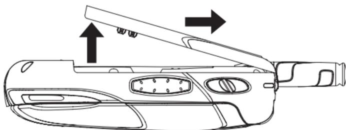
4. Insert the top of the battery into the battery area. Be sure the gold-colored areas on the battery and on the phone are touching.
