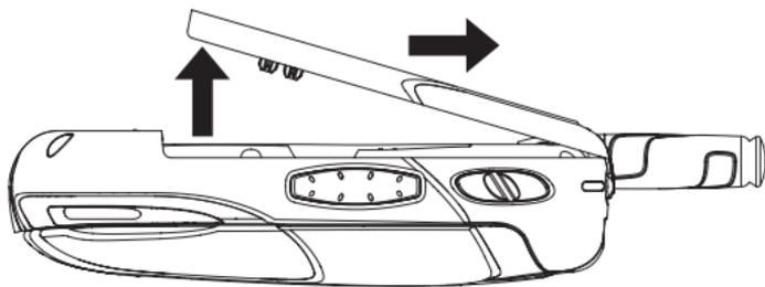
4. Remove the battery by lifting it out from the side.
