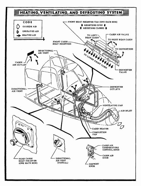
which shuts off the heater when the duct temperature reaches approximately 220°F. When the duct temperature drops to a normal operating level, the heater will restart automatically. The action of this switch is independent of the cabin thermostat setting, and it is not adjustable in flight.
