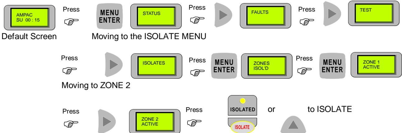
Zone 2 accessed and ISOLATED - To DE-ISOLATE press the ISOLATE or DOWN button.
