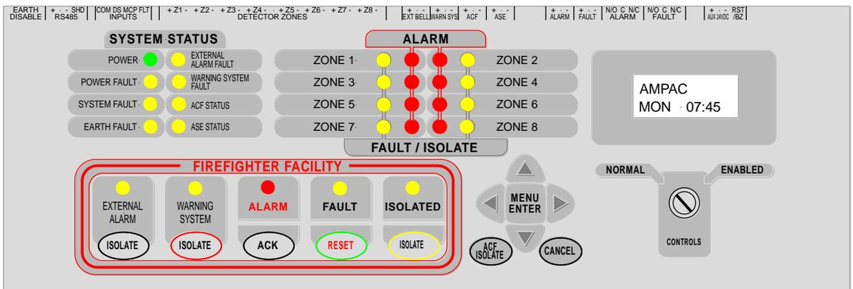
Figure 1: AS4428 8 Zone Front Panel Controls and Indicators
