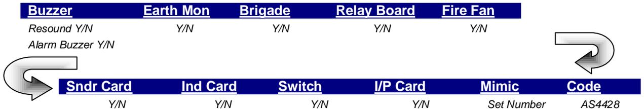
**Buzzer** is the only option that has a sub-menu where the operator is required to make a selection from the options offered.
