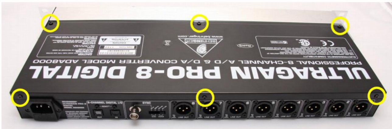
Picture 4: Remove the top cover (6 screws, different sizes!)
