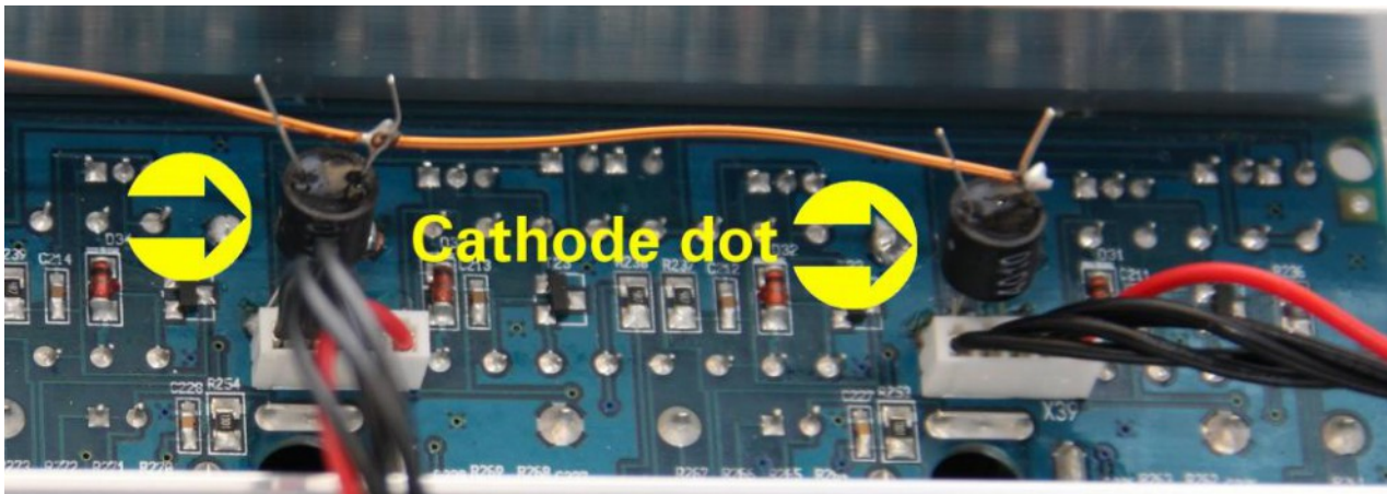
Picture 11: Coupler wiring
