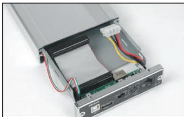
2. Before installing the hard disk in the enclosure, please check your hard disk interface type. To install the SATA hard disk you need to exchange the power and data cables (included). PATA is the default configuration.
