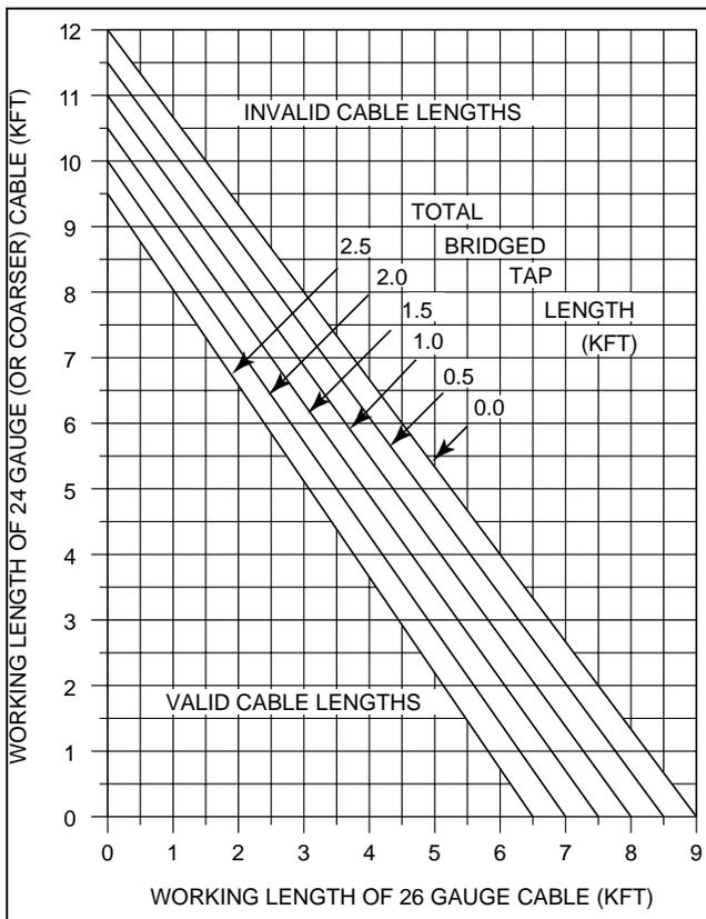
**Figure 43. HDSL2 Deployment Guidelines**
