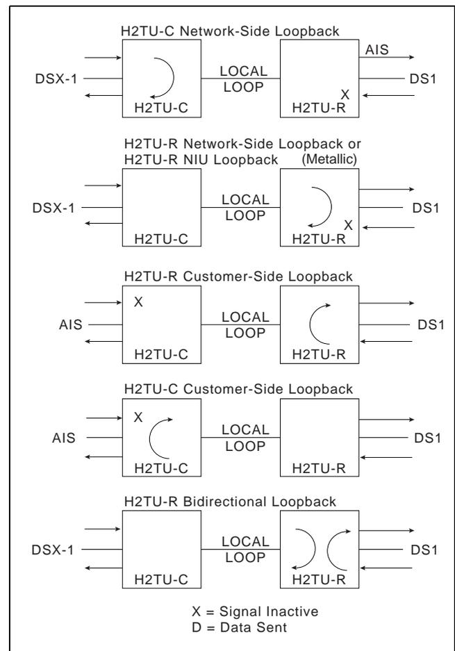
**Figure 6. HDSL2 Loopbacks**
