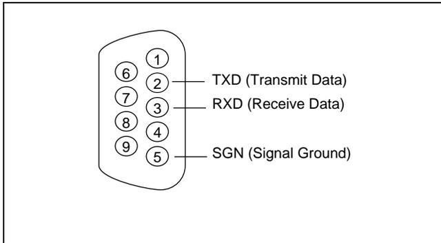
**Figure 7. RS-232 (DB-9) Pin Assignments**
