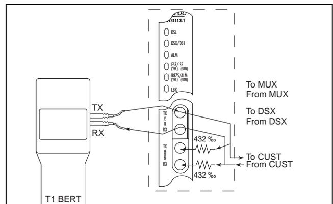
Figure B-3. DSX EQ, Tx to Customer, RX from Customer
