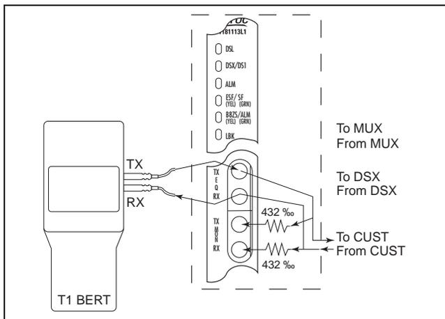
**Figure B-7. MUX EQ, TX to Customer, RX from Customer**
