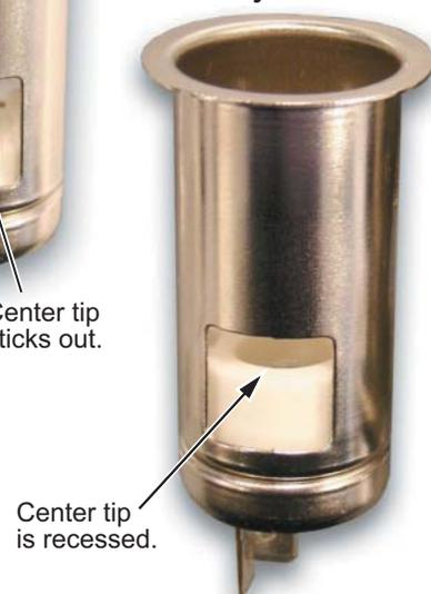
To fix this problem, check to see if the power socket has a center tip that sticks out. If it does, then replace the power socket with P/N 39624-SZ3-L01, H/C 8445454, and replace the fuse. This new style power socket has a recessed center tip that doesn't cause the power adapter to short when you plug it in. If the power socket already is this new type, then look for other possible causes for the blown fuse.
