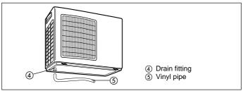
To drain the condensate water to a drain while operating in heating mode, insert the drain fitting into the hole underneath on the left of the base and use a vinyl pipe with a 16 mm internal diameter. It must not be used at temperatures lower than 0°C. (not supplied for low temperature versions).
