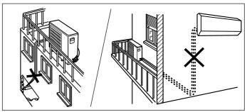
Excessive height difference between indoor and outdoor unit (see Table II "Connections"). Excessive distance between indoor and outdoor units. (see Table II "Connections").
