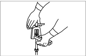
Remove flare nuts from the unit connections and place them on the tube end.
