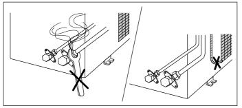
Disconnecting the refrigerant connections after installation: this will cause refrigerant leaks.
