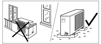
Any obstruction of the unit air outlet and intake or any obstacle that is too close (see minimum clearances required). Installation on grassy ground or soft surfaces (in these cases a solid foundation must be included).
