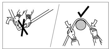
Flattening or kinking of refrigerant or condensate pipes.
