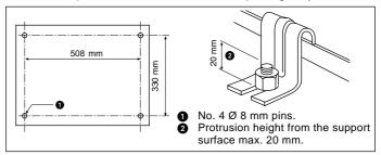
Fix the unit with locally purchased bolts buried in the block to prevent overturning due to strong gusts of wind.
