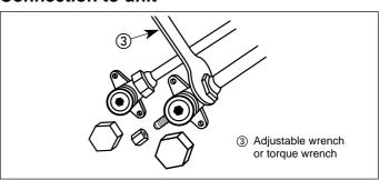
Insufficient tightening torque will cause gas leaks. Overtightening the fittings will damage the tube flaring and cause gas leaks.
