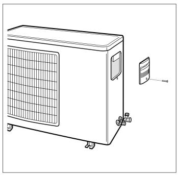
Make refrigerant connections before electrical connections.
