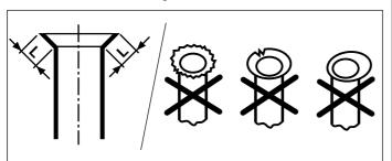
Flare end must not have any burrs or imperfections. The length of the flared walls must be uniform.
