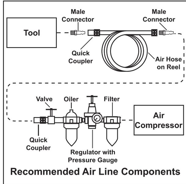
To extend the life of your air tools and equipment, install an oiler and water filter in series with the Air Outlet Valve (4) of the Air Compressor.
