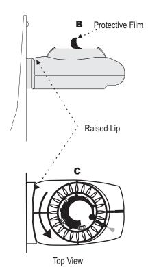
Ensure that controller knob is fully rotated counterclockwise to the OFF position prior to plugging controller into grill and outlet.
