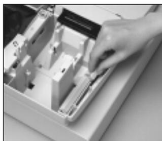
2. Remove the battery compartment cover. Pressing down where the cover is marked "
