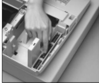
3. Note the (+) and (-) markings in the battery compartment. Load a set of three new SUM-3 ("AA") batteries so that their positive (+) and negative (-) ends are facing as indicated by the markings.
