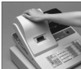
1. Remove the printer cover and inner cover.
