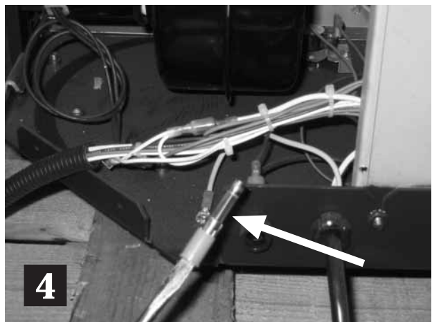
Main fuse (6 AMP quick blow) on back of pellet appliance
