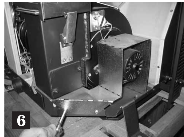
Unbolt blower heat shield (large inserts)
