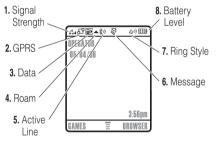
1 Signal Strength Indicator – Vertical bars show the strength of the network connection. You cannot make or receive calls when in the call the call that the call the call that the call that the call that the call that the call
