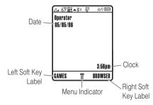
The *menu indicator* shows that you can press to open the menu. *Soft key labels* show the current soft key functions. For soft key locations, see page 1.
