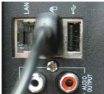
Plug Mouse into USB port
