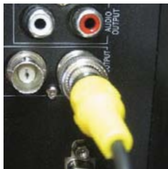
Plug RCA cable to Video Output
