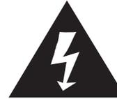
The lightning flash with arrowhead symbol, within an equilateral triangle, is intended to alert user to the presence of uninsulated "dangerous voltage" within the product's enclosure that may be of sufficient magnitude to constitute risk of electric shock to persons.
