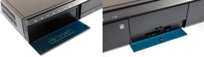
Please pull down the cover from left side of the player, then install HDD into mobile rack.
