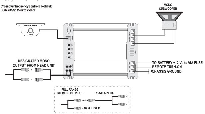
Note: You can use the Radio/CD designated mono line output or a full range stereo line output. For full range stereo line output, you will need an optional "Y-Adaptor" as shown
