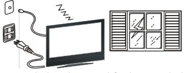
**Power Lines** - An outside antenna system should not be located in the vicinity of overhead power lines or other electric light or power circuits, or where it can fall into such power lines or circuits. When installing an outside antenna system, extreme care should be taken to keep from touching such power lines or circuits as contact with them might be fatal.
