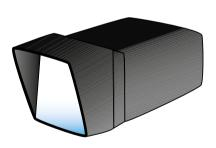
Look on the detector housing for a label\* stating which specification applies. Equipment is approved against MCE 0114 (C), TR 2147, or the current TR 2504. The detector housing may be fixed to the top of the signal head; others are fitted below the head.
