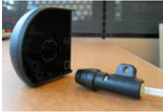
End cap with Home Switch Collar exploded
